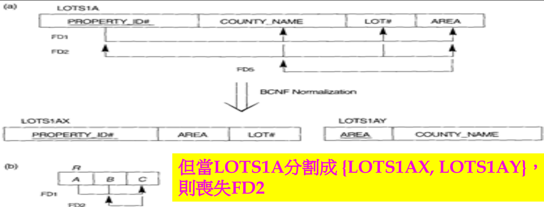
Figure 14.12 Boyce-Codd normal form. (a) BCNF normalization with the dependency of FD2 being “lost” in the decomposition. (b) A relation R in 3NF but not in BCNF.
